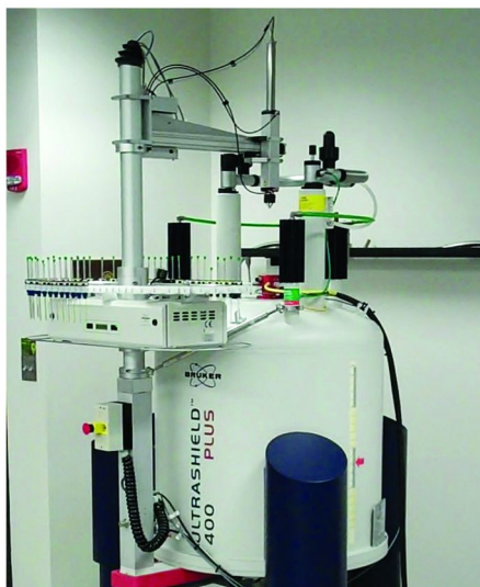
Figure 2. The superconducting magnet and BACS sample changer for the Bruker Avance III NMR.
